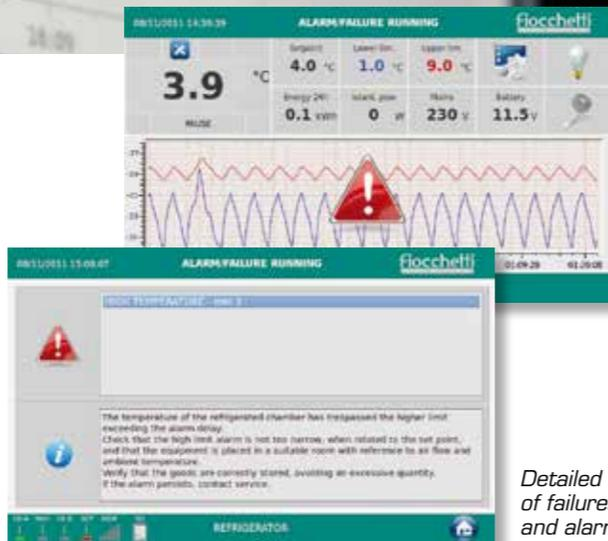
Detailed log of failures and alarms.
