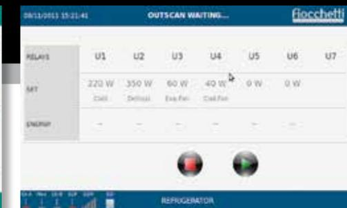
Automatic monitoring of power tension and electric loads.
